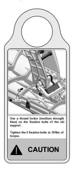
Ski / Spindle assembly bolts must be tightened according to requirements (torque 30 Nm + thread locker).
